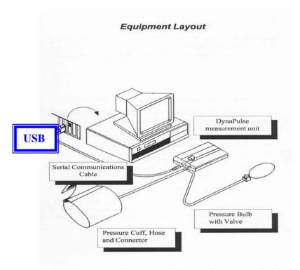
Equipment Layout - Shown a DP-200M monitor connected with a cuff assembly and to a PC's USB communication port
